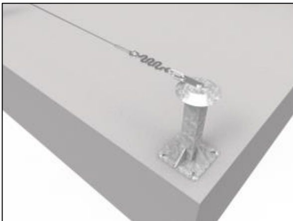
Installation of an energy absorber (F-L-101) and a terminal (F-L-201) on an ANCREE post
